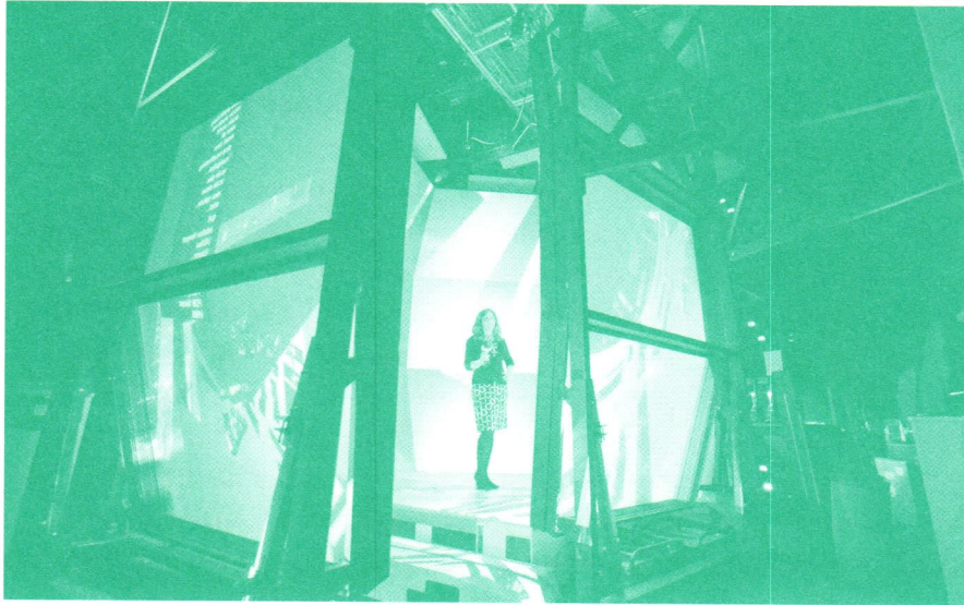
[fig. 1] Dr. Edelstein stands within ... the virtual reality StarCAVE at Calitz, University of California, San Diego. Full-scale 3D models are viewed ... from a first-person perspective, ... allowing designers to analyze ... sight-lines and views with greater ... accuracy, while head-tracking is ... used to evaluate circulation. The ... synchronous measurement of EEG ... brainwaves tracks wayfinding and ... visual attention to design details. ...
